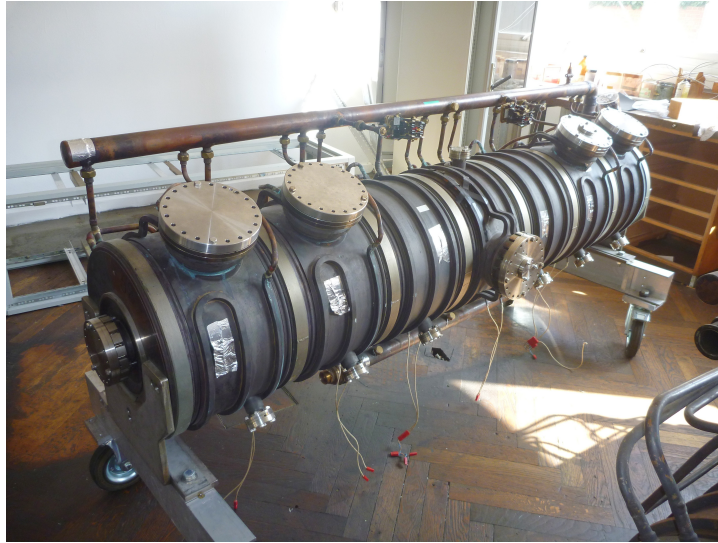
Figure 3.5 – Photograph of a PETRA seven cell cavity. [DES15]
