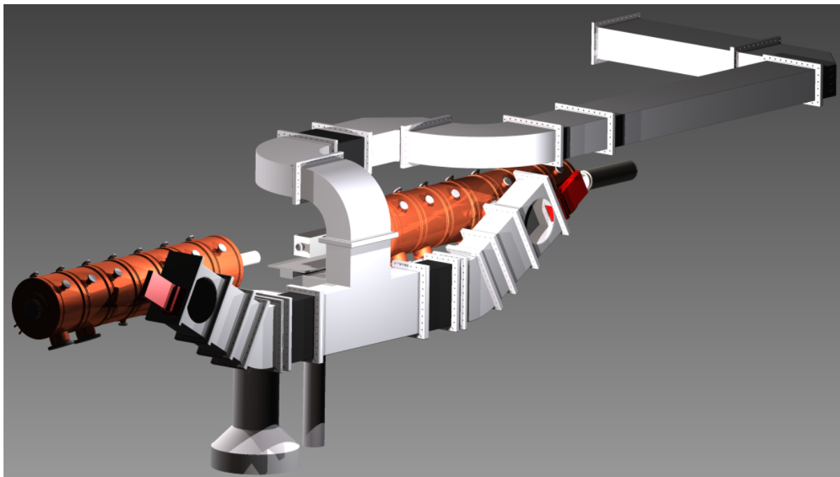
Figure 3.11 – Planed setup for the waveguide transition of the new RF-station. (P. Hänisch)
